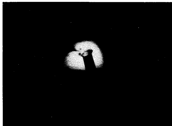
Fig. 14 Forebody vortices at station 1, \alpha = 50 deg, \beta = 5 deg, \phi = 0 deg.
