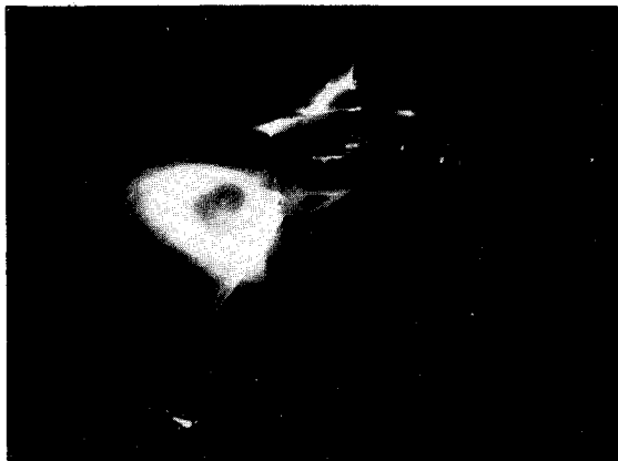
Fig. 11 Strake (LEX) vortices at station 10, \alpha = 30 deg, \beta = 0 deg, \phi = 30 deg.
