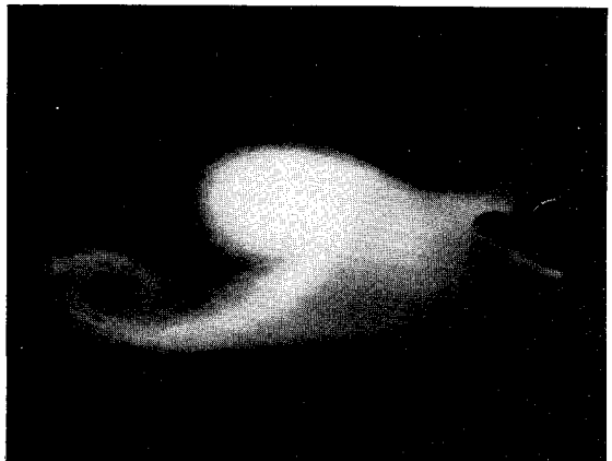
Fig. 8 Strake (LEX) vortices at station 8, \alpha = 55 deg, \beta = 0 deg, \phi = 30 deg.
