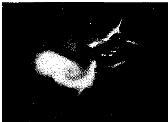
Fig. 12 Strake (LEX) vortices at station 10, \alpha = 35 deg, \beta = 0 deg, \phi = 30 deg.
