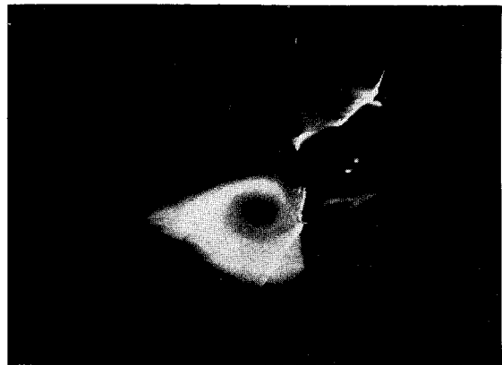
Fig. 13 Strake (LEX) vortices at station 10, \alpha = 40 deg, \beta = 0 deg, \phi = 30 deg.
