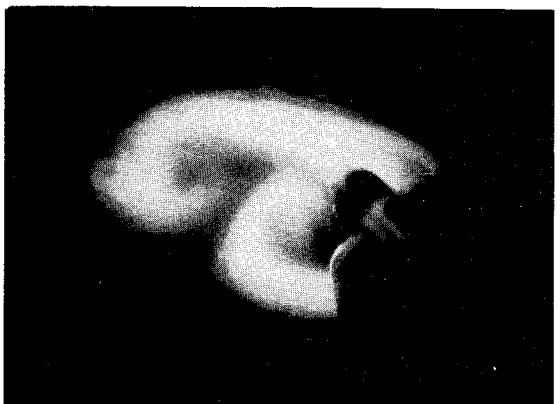
Fig. 9 Strake (LEX) vortices at station 8, \alpha = 55 deg, \beta = 0 deg, \phi = 45 deg.
